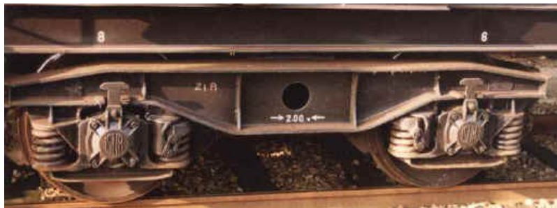
Welded bogie Y 21, wheelbase of 2.00 m, 920 mm wheels, visible mostly in tanks, etc ...
