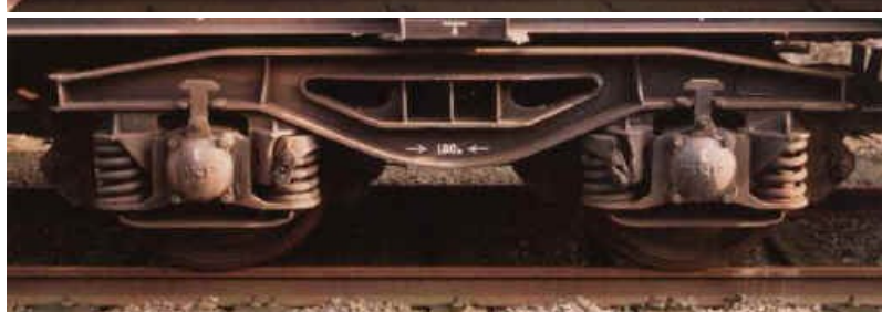
Welded bogie Y 25, wheelbase of 1.80 m, it is THE most used truck today. Wheel diameter 920 mm.
