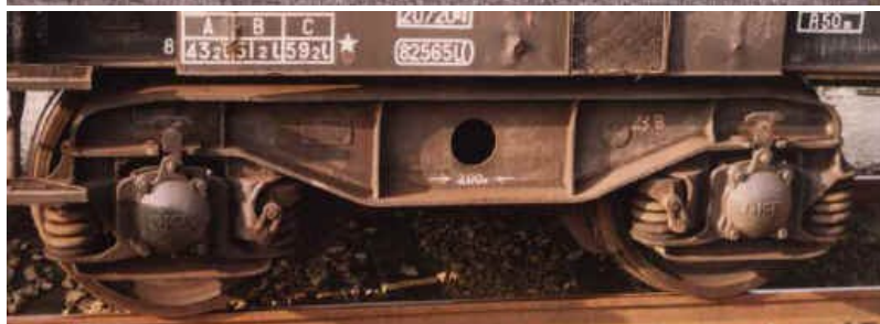
Welded bogie Y 23, wheelbase of 2.00 m, 920 mm wheels, visible mostly in tanks, etc ...
